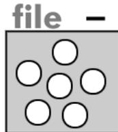
If the filename does not end with any of the designated stencil factor marks, then it is a nested design, which is not normally compatible with jet cutting (plasma, laser, waterjet), but it works for vinyl cutting, engraving, routing and processes that have backing material or that do not cut all the way through.
