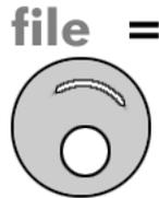
**~ Tilde Sign** means the design is a copy of the above form, except some thin details are converted to centerlines (cut starts at one end and stops at other end) Enables plasma to cut the same design smaller. Not normally compatible with vinyl cutters, but with low knife pressure such lines can be scribed in the vinyl without cutting through, which can make it possible to vinyl cut at extremely small scale.
